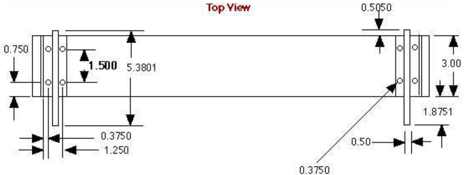
Dimensions for Machining the Main Base
